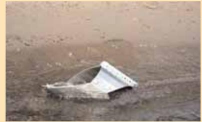
The pictures show another type of the patented Moorsafe anchor concept, which is designed to be used as a ship anchor. Picture 1 to 6 show, that even if the wind changes direction by 180° the Moorsafe ship anchor will turn around and correct itself and quickly penetrate the seabed again.
